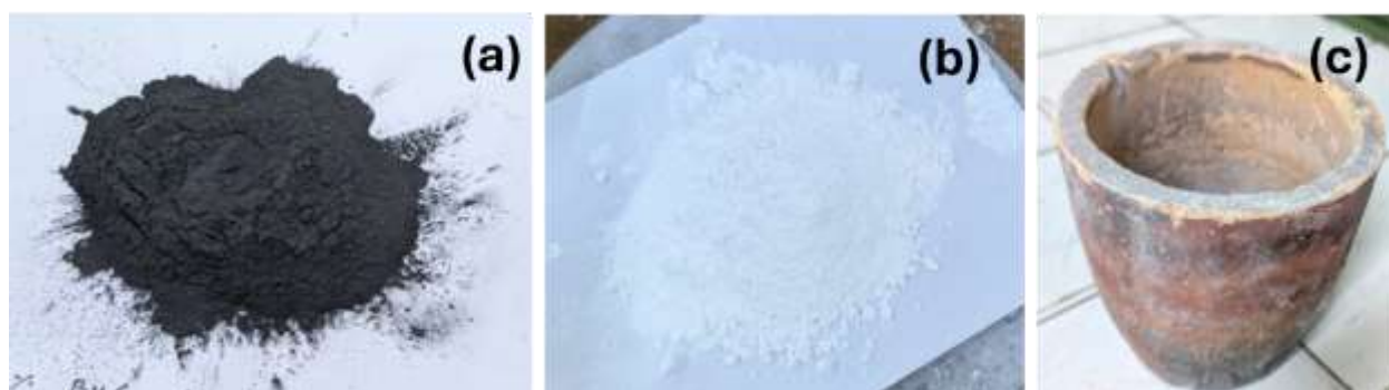
Fig. 1(a) Boron Carbide Powder, (b) Titanium Dioxide Powder, (c) Ceramic crucible.
