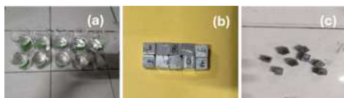
Fig. 3(a) Sample in NaCl solution, (b) Samples for corrosion test, (c) Samples after corrosion test.
